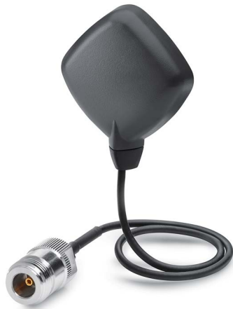
Figure A-4 GPS antenna, ANT895-6ML, flat antenna
